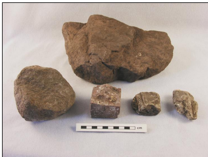
Figure 15. Architectural Materials At Behavior. Top, bottom left, micaceous feldspathic sandstone; center gneiss; right impressed tabby. From Feature 1, FS 15.
